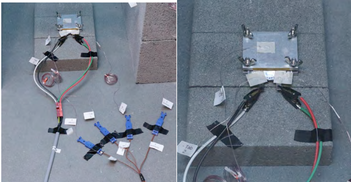
Figure 13: Overcharge cell test set-up performed at Exponent.
