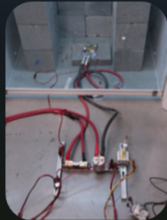
No thermal runaway even when cell is short circuited
